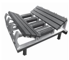
Rulmeca presents a new product to widen the range of components for belt conveyors: impact bars used at the loading point of the conveyor under the hopper. These impact bars utilise the important properties of two materials such as the low friction of polyethylene and a quality rubber to absorb shocks.
