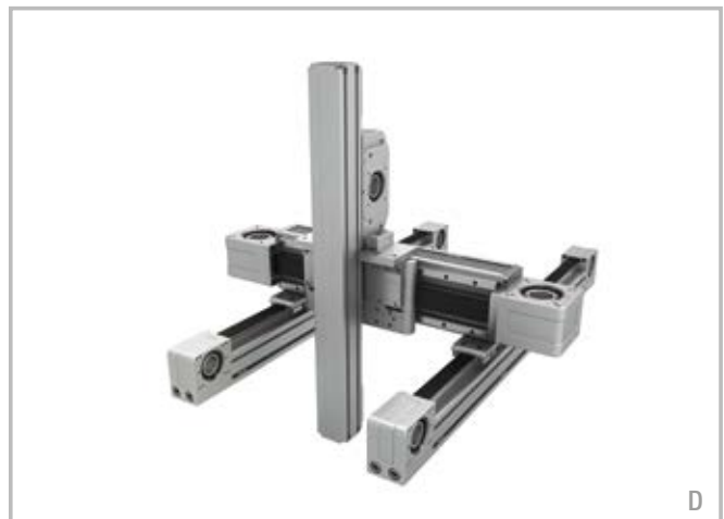
D - Linear units: X Axis 2 E-SMART - Y Axis 1 R-SMART - Z Axis 1 S-SMART Connection kit: 2 fixing brackets Kit for 2 R-SMART (Y axis) on 2 E-SMART (X axis). Connection plate Kit for S-SMART (Z axis) on 2 R-SMART (Y axis). Parallel Kit
