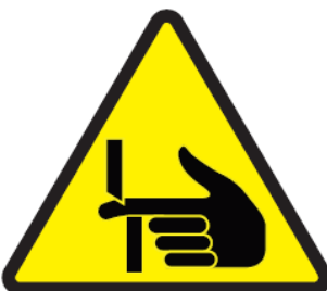
Crush hazard at bottom valve
