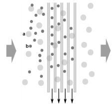
Aerosols when passing through the separation plates
